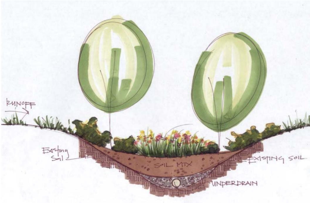
*Section illustrating basic components of a raingarden*
